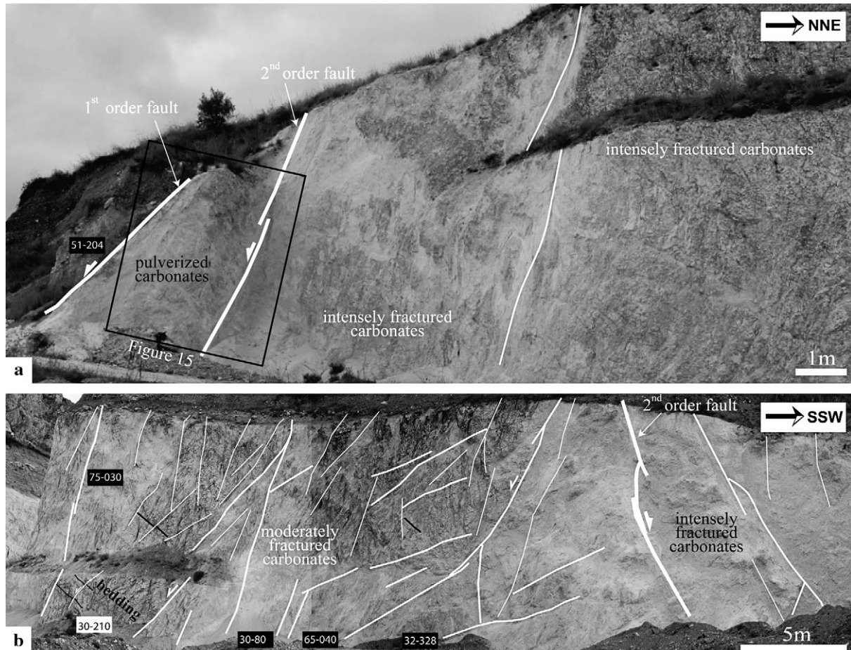
Fig. 5. Sections of the nearly vertical walls of the Santilli Quarry that are oriented orthogonal to the first-order fault strand. The trace of the second fault strands (white thick mark), and third order fault strands with more than 5 cm offset (white mark) are shown. The bedding is denoted with a black mark. (a) Outcrop #1, (b) outcrop #2, (c) outcrop #3, (d) outcrop #4.
